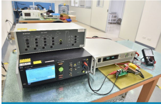
EFT & Surge Immunity Test Station
