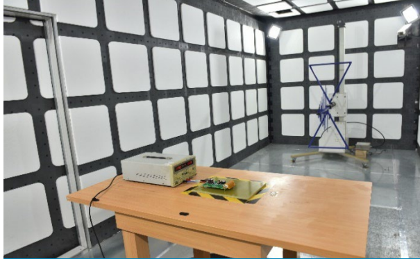
Radiated Emission Test Station
